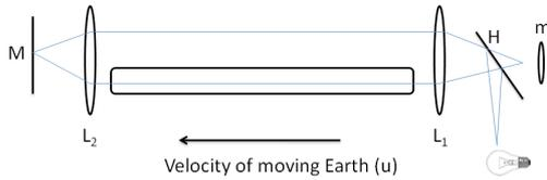
Fig.8. Optical set up of Hoek’s experiment on the optics of moving media.  $L_1$  and  $L_2$  are converging lenses; H, half-silvered mirror; M, mirror; m, microscope with micrometer.
