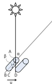
Fig.6. Refraction through a water-filled telescope. The star is shown directly overhead in its “present” position.
