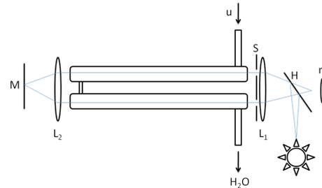
Fig.7. Fizeau's experiment on the propagation of light through moving water. m, microscope with micrometer; H, half-silvered mirror; L<sub>1</sub>, L<sub>2</sub>, converging lens; S, slits; M, mirror.
